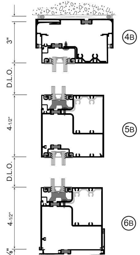
Shown with shear clips. Screw spline assembly similar without clip. OUTBOARD PLANE - OUTSIDE GLAZE
