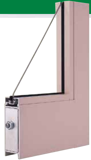
Modified Narrow Stile 1-3/4" x 2-1/8" Door with 4" Bottom Rail; BP Beige Painted Finish, 1/4" Glass
